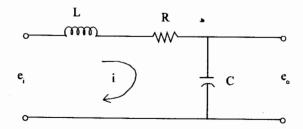
(c) Explain force-voltage analogy, of translational mechanical system. Draw the analogous electrical system.
